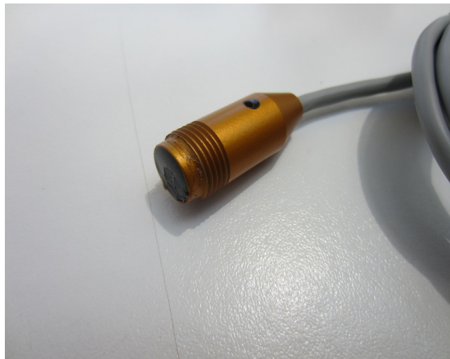
Image of the sensor body. It screws into the sensor body. The body contains the sensor and a small micro processor used to linearise the flow reading derived from the vortex suspended rotating object in the sensor housing.
