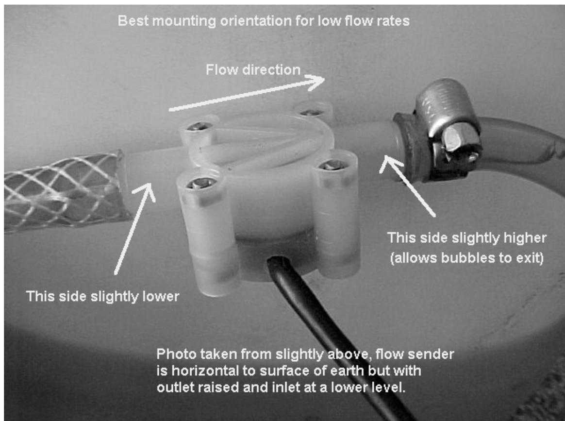
For installations where long fuel lines are unavoidable we recommend to fit the fuel flow sender AFTER the fuel pump. Install a second fuel filter before the sender to act as reservoir to prevent pressure pulses from the fuel pump to affect the fuel flow reading accuracy.
