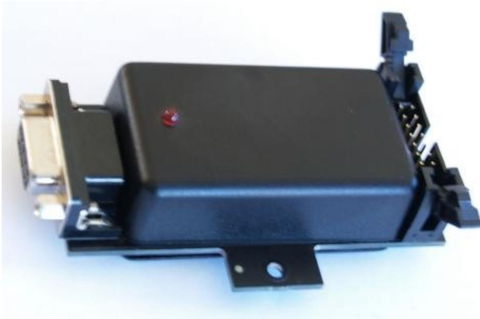
The CNV-AT converter accepts the altitude and local pressure setting information from the airtalk link and converts this information to Gillman code in a format compatible with mode-C transponders.
